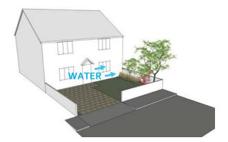
Non permeable surfacing may cover part of the front garden, providing that surface water is directed onto a porous or permeable surface, such as a grassed area
