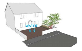
Driveway / hardstanding is constructed from porous or permeable material
